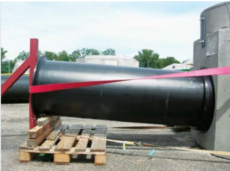
FIG. 9: Test of an inspection chamber connection d 630mm
