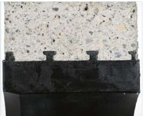
FIG. 10: The undercut anchoring webs of the inspection chamber lining ASF provide a strong and tight connection to the concrete
