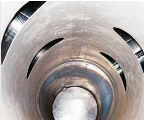
FIG. 16: Detail of the test set-up with four FRIAFIT sewage saddles before burying
